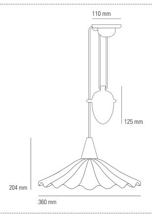
Cable length may be shortened upon installation. This will reduce both maximum & minimum drop and reduce the range of movement.
